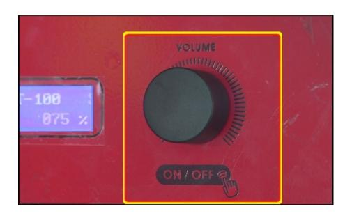
**Step 6:** To stop or pause the flow of fog, press the "VOLUME" rotary dial once. To resume the flow of fog, press the "TIMER" rotary dial once
